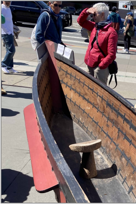
Bow of the ti'aat. The stem is angular. Chumash tomols have rounded stem or prow.
